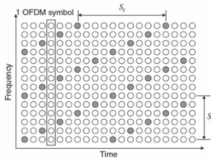
**Figure 2(c).** Lattice type structure [2].
