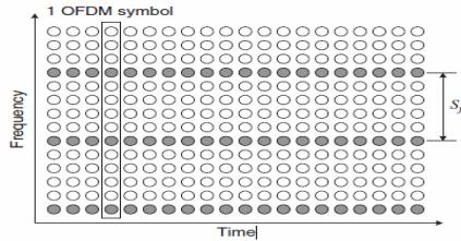
**Figure 2(a).** Comb type structure [2].
