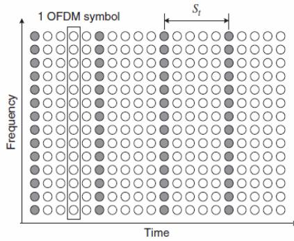
**Figure 2(b).** Block type structure [2].
