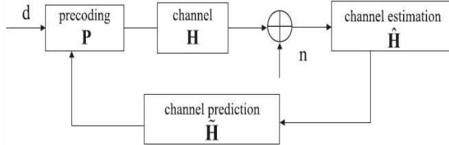
**Figure 3.** Predicted precoding channel estimation multi-user (MU)-MIMO-OFDM system [1].
