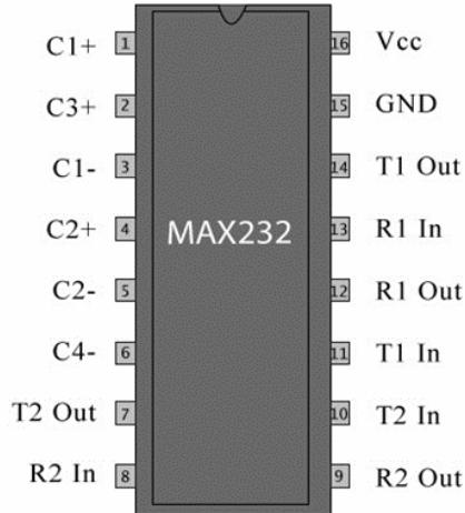
**Figure 4.** Pin diagram of MAX232.
