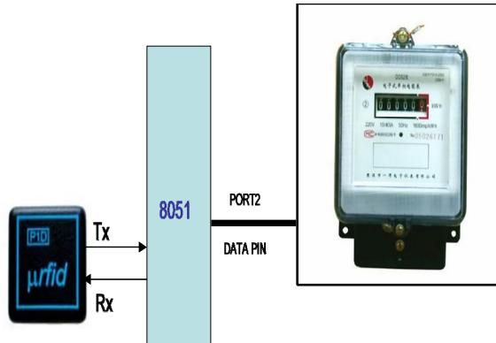
**Figure 5.** RFID interfacing with a microcontroller.
