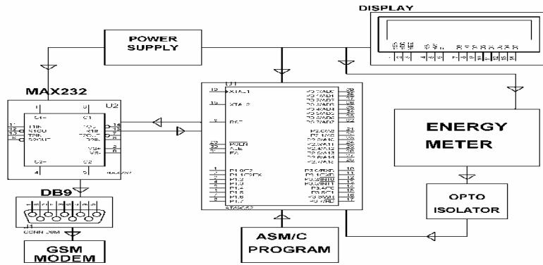
**Figure 1.** Block diagram using opto-isolator.
