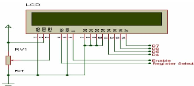
Figure 3. Pin diagram of liquid crystal display.
