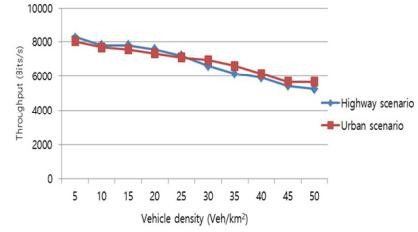
**Figure 4.** Throughput vs vehicle density in LTE.
