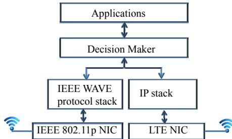
**Figure 1.** Protocol layers used in heterogeneous VANET.
