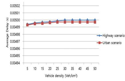
**Figure 6.** Delay vs vehicle density in LTE.
