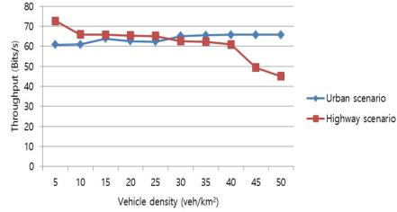
**Figure 3.** Throughput vs vehicle density in 802.11p.
