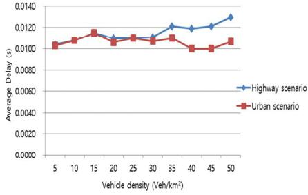
**Figure 5.** Delay vs vehicle density in 802.11p.
