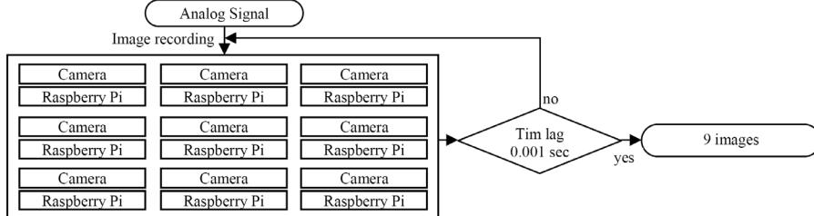
**Figure 1.** Synchronization recording algorithm.
