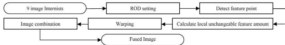
**Figure 5.** Image fusion algorithm.
