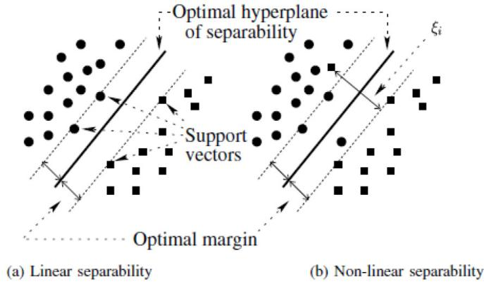
**Figure 1.** Linear separable classes; right: nonlinear separable classes. Measures the error of the fitting hyperplane [11].
