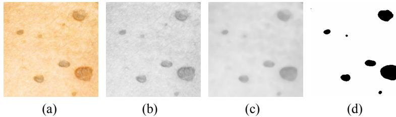
**Figure 4.** Experiment images (a) RGB image (b) grayscale image (c) noise reduction with median filtering (d) binarization image with Otsu's algorithm.
