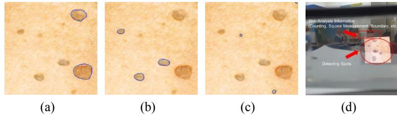
**Figure 5.** Detecting spots with  $K$ -means (a) large size spots (b) medium size spots (c) small size spots (d) projected in the space with AR HMD.
