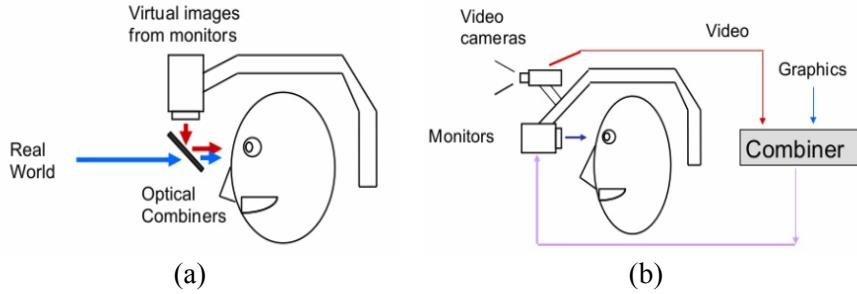
**Figure 1.** AR HMD system (a) optical see-through HMD (b) video see-through HMD [3, 6].
